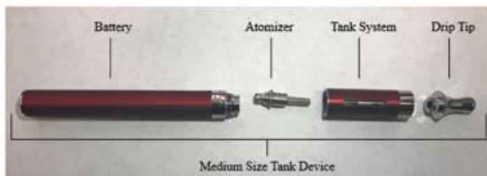
Figure 1. An example of an ENDS device and its parts and components.
